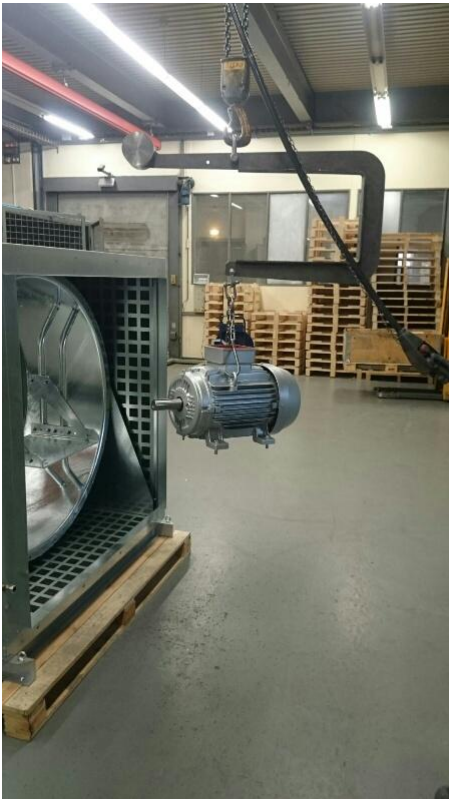
Fig 21 Typical motor lift for Long case axial
